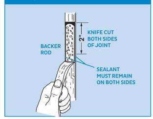
5. Sealant may be replaced by applying more sealant in the same manner as it was originally applied. Care should be taken to ensure that the new sealant is in contact with the original, and that the original sealant surfaces are clean, so that a proper bond between the new and old sealant will be obtained.
